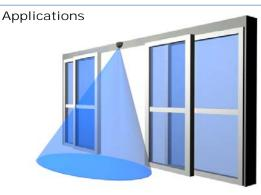
The Eagle's flat antenna provides a stable detection that can detect people approaching the door from odd angles.
